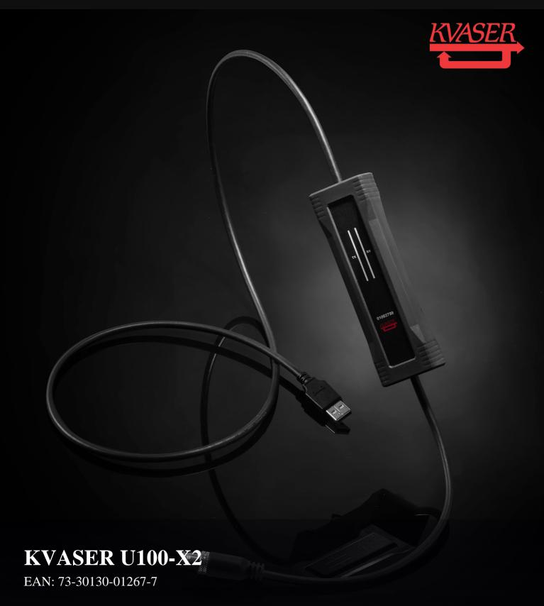
The Kvaser U100-X2 is a robust, single-channel CAN/CAN FD to USB interface with reinforced galvanic isolation that squarely addresses the needs of the evolving automotive development market. Fully compatible with J1939, CANopen, NMEA 2000® and DeviceNet, this is the first in a new range of interfaces that is also suited to rugged applications in marine, industrial, heavy duty vehicle and heavy industries.
