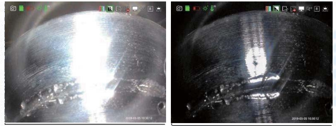
Exposure Setting: exposure suppression--the polished object is also inspected clearly; exposure compensation--when checking large cavity, it can be more effective and clearer
