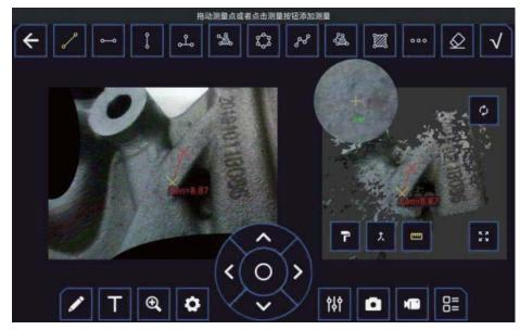
Click the section key in the upper tool area to view the section depth of the area to be inspected on the left.
