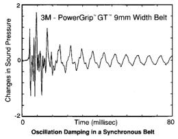
to the microcomputer inside the Sonic Tension Meter for processing and conversion into the natural frequency. To calculate belt tension, the Sonic Tension Meter system uses the "transverse vibration of strings theory." To operate the meter, the belt mass, span length and width of the belt must be entered.
