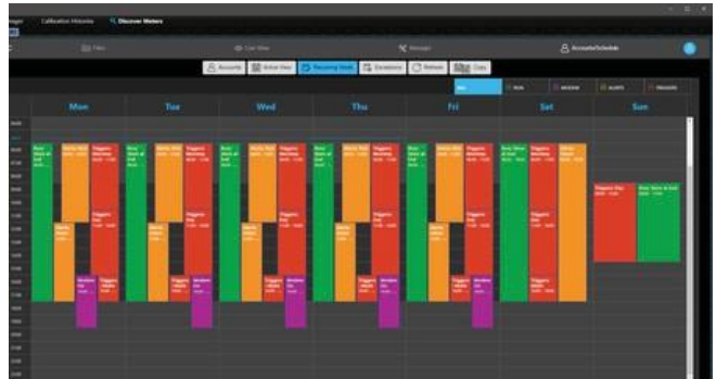
Example of an 831C-SCH schedule with daily Run/Save times (green), two alert recipients on weekdays (orange), three alert levels (red), a special weekend schedule, and the modem "waking up from" low power consumption mode every weekday evening (purple).
