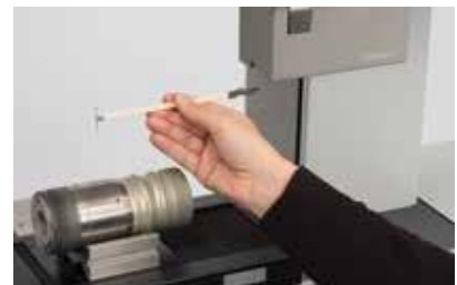
Probe arms with magnetic coupling
