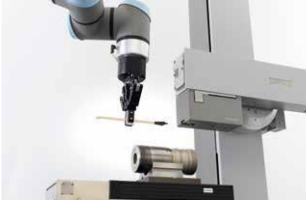
Probe arm change via robot – magnetic holder
