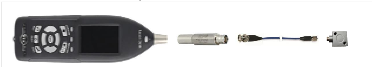
FIGURE 19-1 Example Connection: 831C, ADP074, Cable, and Accelerometer
