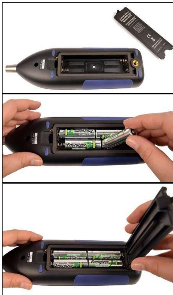
FIGURE 2-3 Installing batteries into the 831C.
