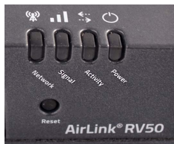
Figure 3-14 Gateway Status Indicators
