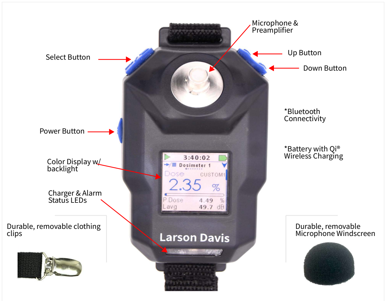
FIGURE 1-8 Components of the Spartan Model 730
