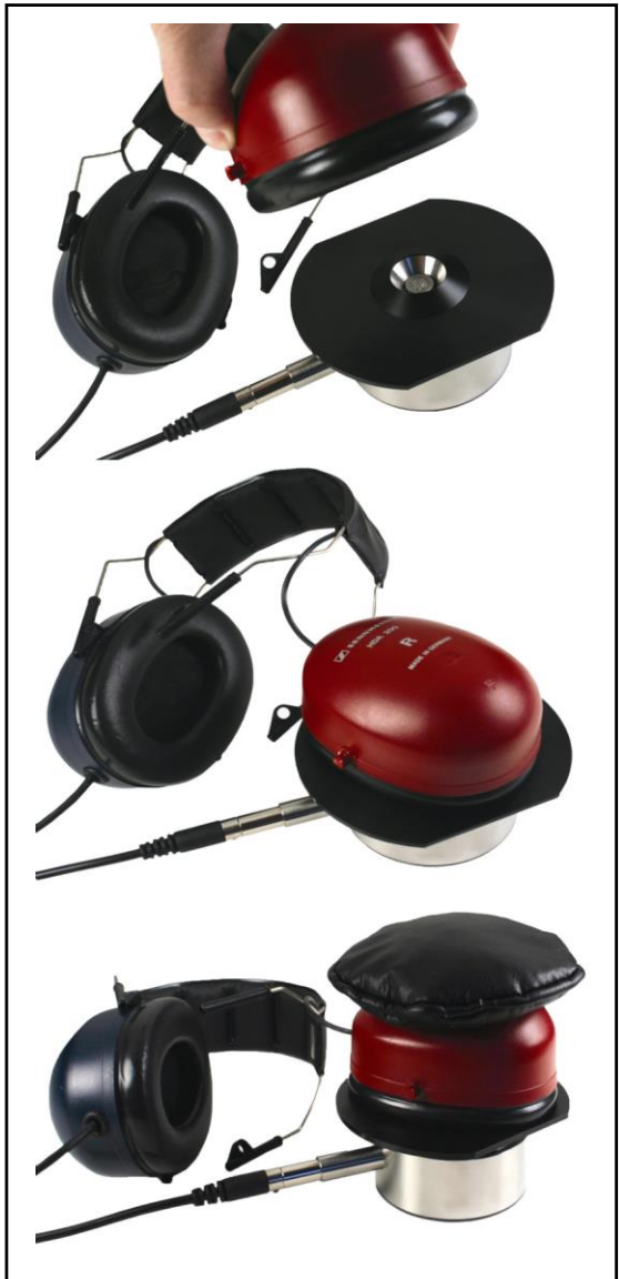
FIGURE 3-7 Sennheiser earphone and weight being installed on AEC201
