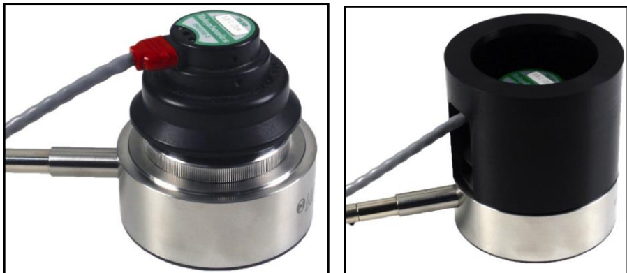
FIGURE 3-3 Earphone and retainer ring being installed on AEC201
