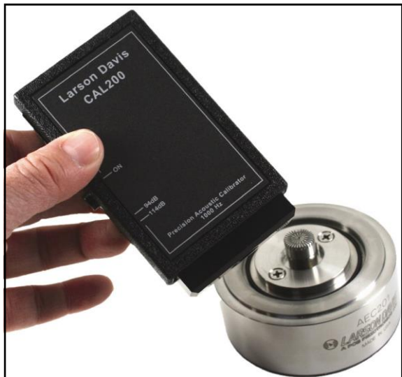
FIGURE 2-4 Installing the CAL200 on AEC201
