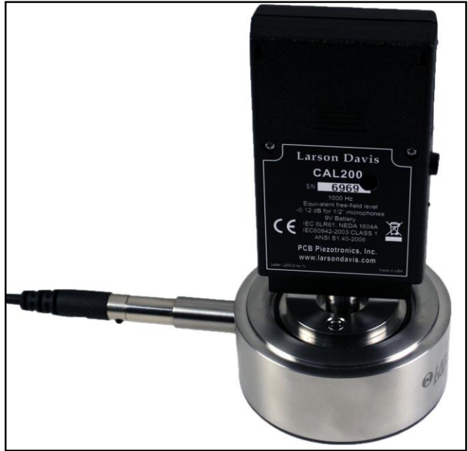
FIGURE 2-5 CAL200 being activated on AEC201
