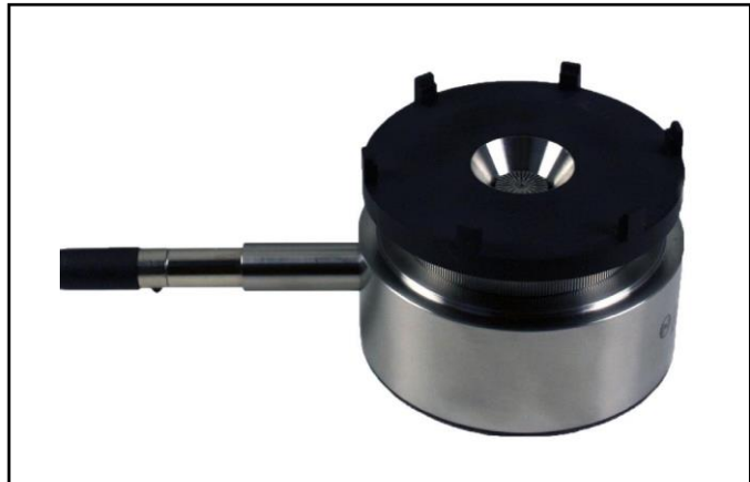
FIGURE 3-6 Type 2 adapter installed on AEC201
