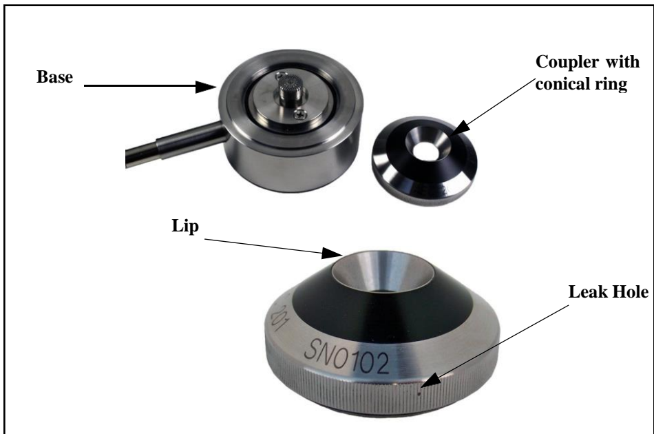
FIGURE 2-1 AEC201 with coupler, leak hole
