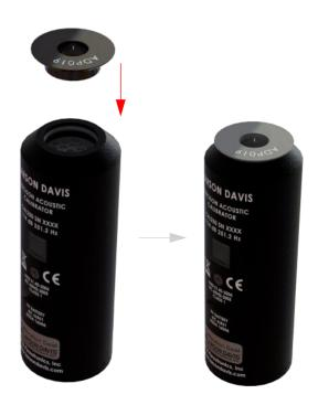
**Step 3** Insert the microphone through the adapter until it is fully seated in the calibrator.
