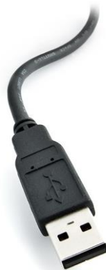
Figure 2: A standard USB type “A” connector.
